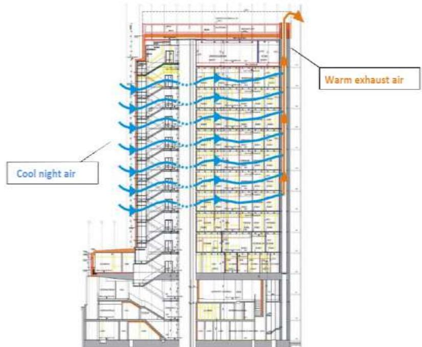
Figure 16 Cooling system TU Vienna Plus Energy building
